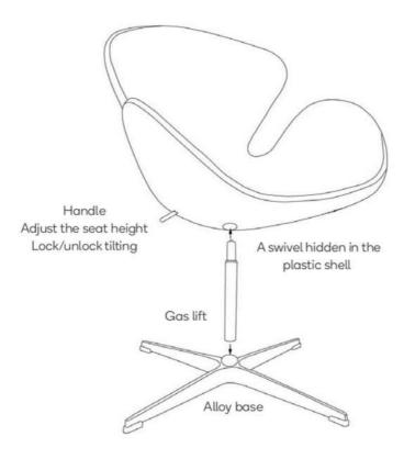
**Handle:** Pull the handle outward when you want the chair to tilt. Push the handle inward to lock the chair to an upright firm position. Do not adjust the handle if the chair is currently occupied.
