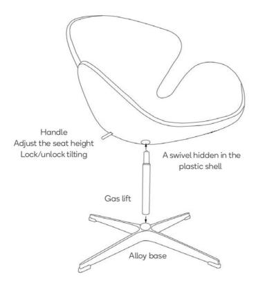
**Handle:** Pull the handle outward when you want the chair to tilt. Push the handle inward to lock the chair to an upright firm position. Do not adjust the handle if the chair is currently occupied.
