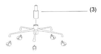
Step 4: Align the Chair Body with the Gas Spring and lower it onto the Base Assembly.
