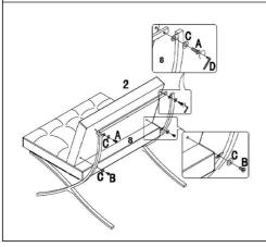
Attach chair back frame (8) with long screw (A) and flat washer (C).
